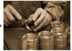
This is the process of polishing and smoothing the surface of metals and glass. This work is also done by the hand of craftsmen in addition to machines.
