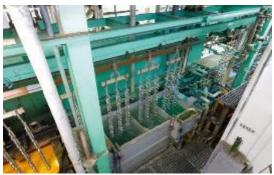
This is the process of covering the surface of metals with film. The purpose of this is to prevent corrosion of the base and to improve the texture of the surface.
